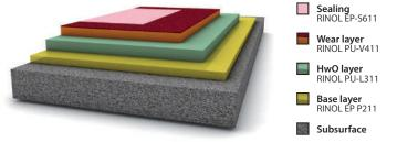
Besides the ramp, the weathered open-air deck of a multi-storey car park represents the greatest stress for the coating system. Besides the most far-reaching congruent requirements of the floor slab and the intermediate deck, here the RINOL OS11a coating system fulfills the protective functions required in extremely different climatic weather conditions.
